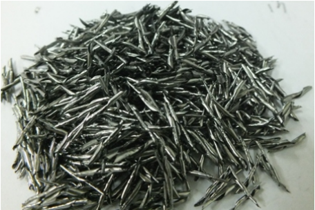
SMOOTH CUTTING GOOD CHIP BREAKING SLIGHT WEAR ON CUTTING EDGE
